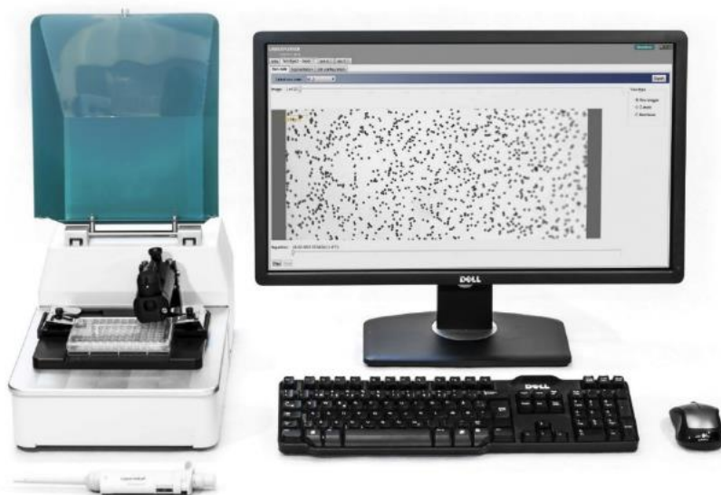
Figure 1 The oCelloScope system consists of the oCelloScope instrument and the UniExplorer software. The instrument has dimensions of 45 × 26 × 25 cm to allow portability and fit inside standard laboratory incubators for biological applications (temperature: 20 – 40 °C, humidity: 20 – 93%).
