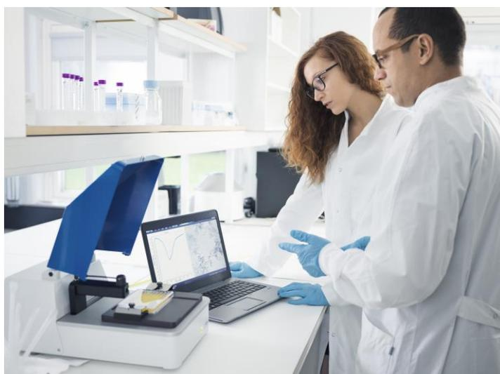
**Figure 2.** Photograph of the open oCelloScope imaging system loaded with a 96-well plate. The dedicated software displays images and curves resulting from a growth experiment performed on samples of *Saccharomyces cerevisiae*.
