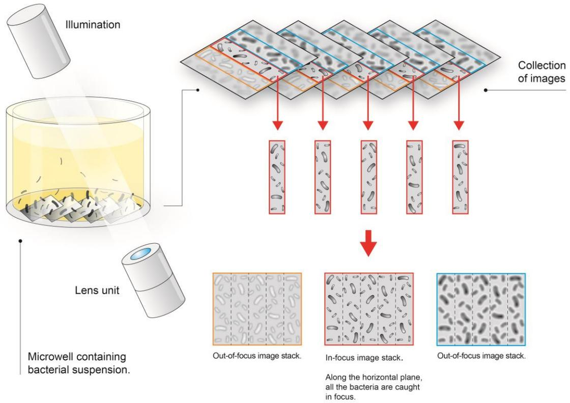
**Figure 2.** Schematic showing the oCelloScope optical scanning technology and image analysis applied to a microwell containing bacteria sedimented at the bottom.
