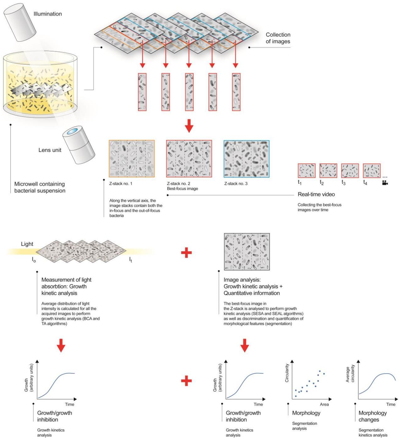
**Figure 1.** Schematic showing the oCelloScope optical scanning technology and image analysis applied to a microwell containing a bacterial suspension.
