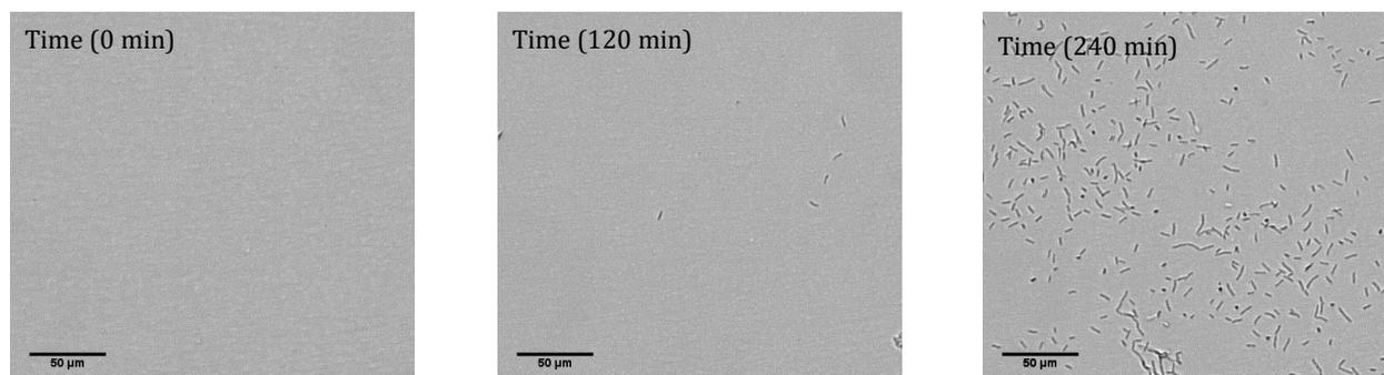
**Figure 2.** Images of the culture from Fig. 1-B at time 0, 120 and 240 minutes. The oCelloScope can detect the growth while the OD plate reader still showed no signal.
