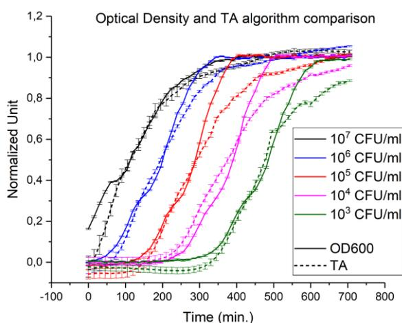
**Figure 3.** *E. coli* growth curves acquired with Thermo-Fisher Scientific VarioSkan (solid line) and with the oCelloScope TA algorithm (dashed line).
